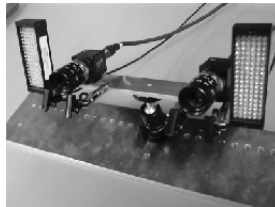
Figure 1. The stereo camera unit our face-tracking system.
